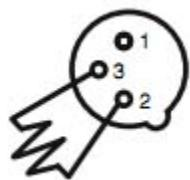
Termination reduces signal errors and avoids signal transmission problems and interference. It is always advisable to connect a DMX terminal, (Resistance  $120\Omega$  1/4 W) between PIN 2 (DMX-) and PIN 3 (DMX +) of the last fixture.
